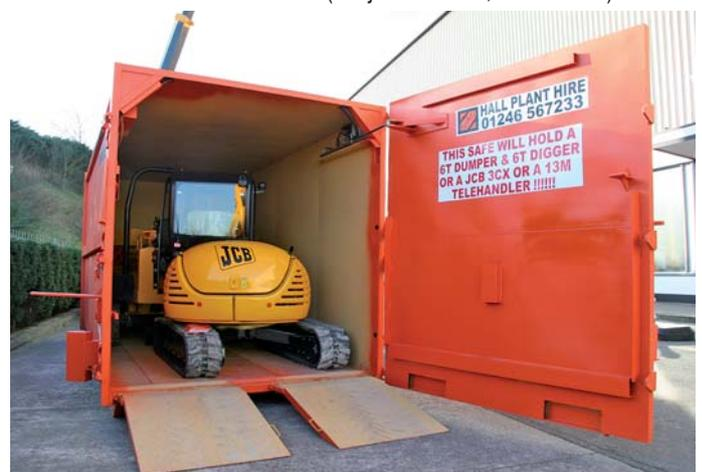
The spacious PlantSafe Maxi can accommodate sizeable items of plant without the need to remove cabs or ROPS frames.
