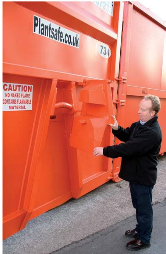
Tim Hall shows off the heavily reinforced steel plate used to hide the hook lift bail bar on the PlantSafe Maxi.
